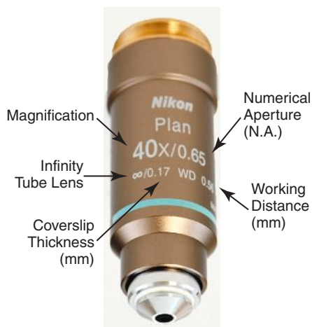
Figure 4-3 Microscope objective lens. The numerical aperture (NA) indicates the light-gathering ability of the objective lens and reflects its ability to distinguish between fine details of two closely situated objects. The working distance (WD) is the distance in millimeters between the lens of the objective and the cover glass when the specimen is in focus. (Courtesy Nikon Instruments, Inc., Melville, NY.)
