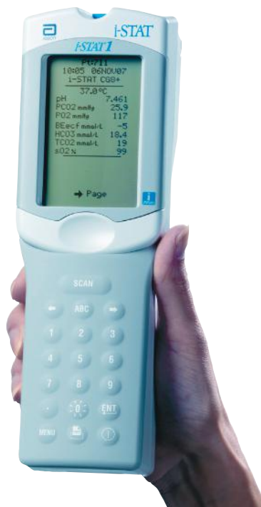
Figure 14-16 i-STAT instrument for measuring hematocrit. (Courtesy Abbott Laboratories, Abbott Park, IL.)
