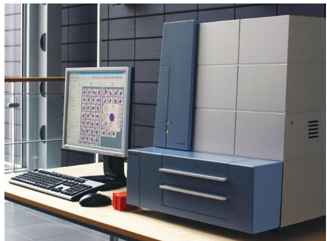
Figure 16-12 CellaVision DM96. CellaVision is an example of an automated system for differential counting that locates blood cells on a stained peripheral blood film, takes digital images, classifies the cells, and presents the cells in the 100-cell differential count to the operator on a computer screen. The operator can override the instrument’s classification and identify cells that the instrument could not classify. (Courtesy of CellaVision AB, Lund, Sweden.)
