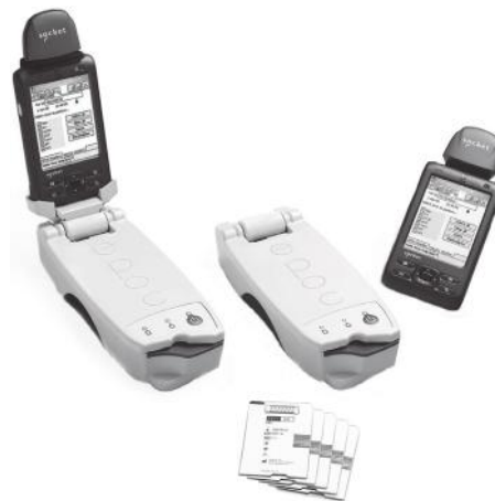
Figure 14-17 Epop device for measuring hematocrit. (Courtesy Epopal, Inc., Ottawa, Ontario, Canada.)
