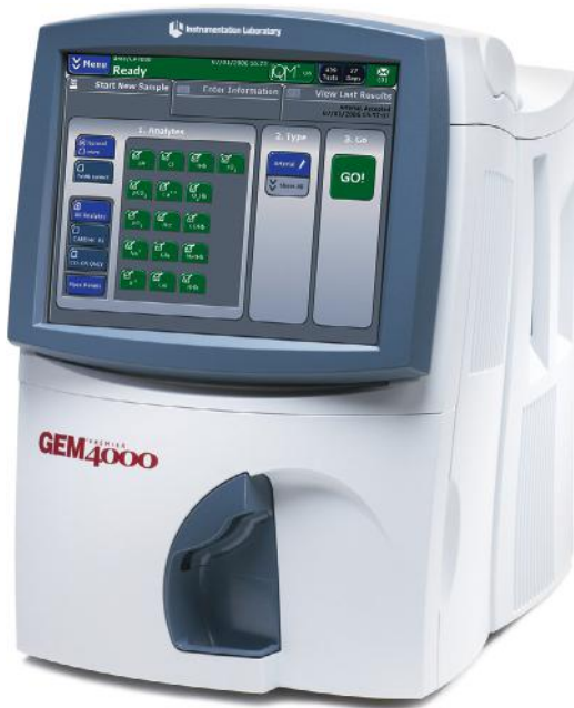
Figure 14-18 Gem Premier instrument for measuring hematocrit. (Courtesy Instrumentation Laboratory Company, Lexington, MA.)
