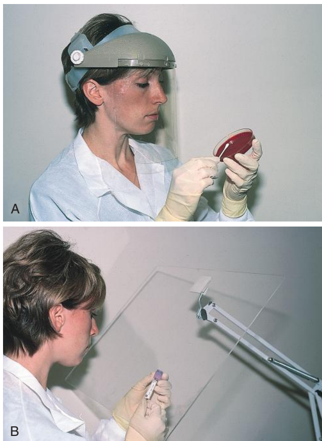
Figure 2-4 Examples of safety shields. A , Face shield. B , Adjustable swing arm shield. (Courtesy Steve Kasper.)
