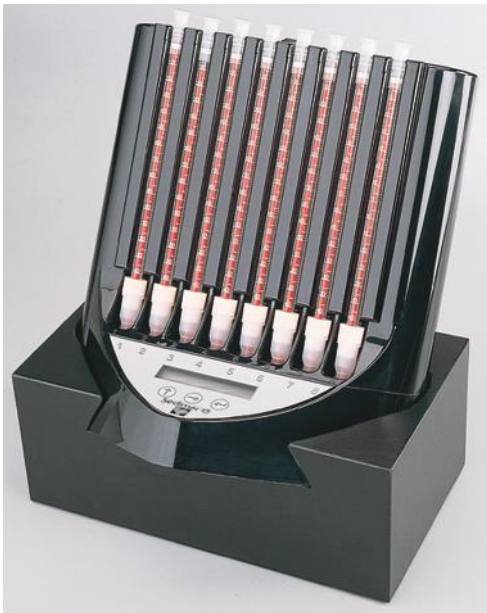
Figure 14-15 Sedimat 15 (Polymedco) automated sedimentation rate system. (Courtesy Polymedco, Cortlandt Manor, NY.)
