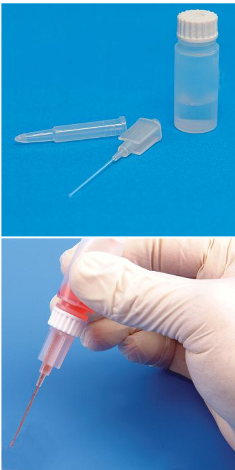
Figure 14-4 LeukoChek™ blood diluting system for manual white blood cell and platelet counts. It consists of a 20 \mu\text{L} capillary pipette and plastic reservoir containing 1.98 mL of 1% buffered ammonium oxalate that makes a 1:100 dilution of whole blood. (Courtesy Biomedical Polymers, Inc., Gardner, MA.)
